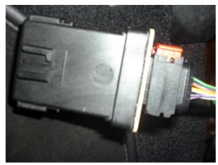
Once you have the unit out you will see a RED clip holding the harness to the 1929SJ Lift this up and gently pull the harness plug off the unit.
